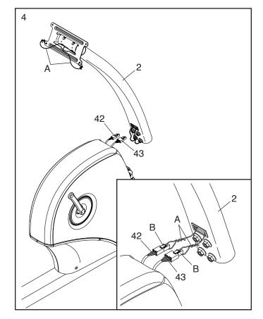
5. **Do not pinch the wires.** Slide the Upright (2) onto the Frame (1).
