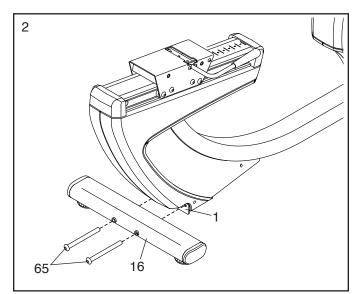
3. Set a sturdy piece of packing material under the front of the Frame (1).
