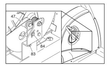
When the drive belt is correctly adjusted, reattach the parts that you removed.
