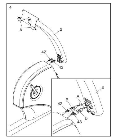
5. **Avoid pinching the wires.** Slide the Upright (2) onto the Frame (1).
