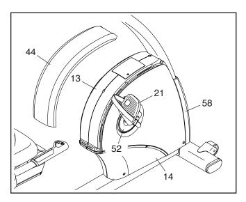
Next, use a standard screwdriver to carefuly pry the Top Shield (44) and the Front Shield (58) off the exercise bike. Next, remove all of the Screws (not shown) from the Left and Right Front Shields (13, 14); **make sure to note which Screw you remove from each hole.** Then, carefully remove the Right Front Shield.
