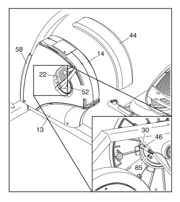
Next, carefuly pry the Top Shield (44) and the Front Shield (58) off the exercise bike. Next, remove all of the Screws (not shown) from the Left and Right Front Shields (13, 14); **make sure to note which Screw you remove from each hole.** Then, carefully remove the Left Front Shield.
