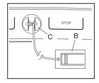
key can be pulled from the console, causing the walking belt to slow to a stop. Test the clip by taking a few steps backward; if the key is not pulled from the console, adjust the position of the clip.
