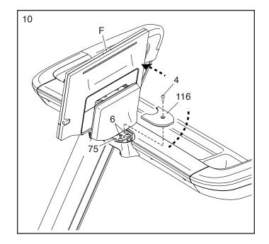
11. Rotate the console assembly (F) to the position shown.
