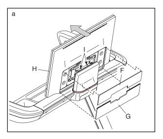
Next, tilt the top of the console (H) in the direction shown by the arrow, and use one of the included hex keys to tighten the two indicated M6 x 15mm screws (I) a small amount.
