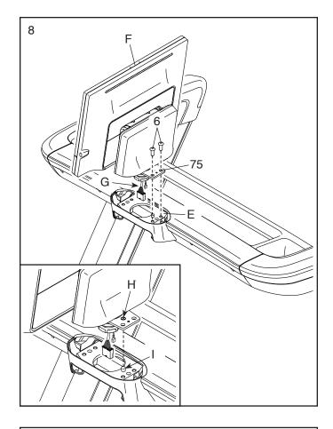
9. Rotate the console assembly (F) so that it faces the opposite direction. Tighten two 5/16" x 3/4" Screws (6) into the Pivot Plate (75); start both Screws, and then firmly tighten them.
