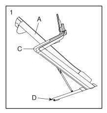
fully move it to the desired location. CAUTION: Do not move the treadmill without tipping it back, do not pull on the frame, and do not move the treadmill over an uneven surface.
