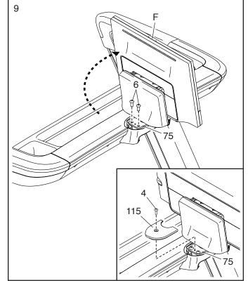
Rotate the console assembly (F) back to its original position. Firmly tighten the two 5/16" x 3/4" Screws (6) that you attached in step 8.
