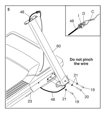
6. Do not pinch the Wires (J, 48) during this step.
