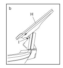
reattach the lower console cover (G) and then the upper console cover (F).
