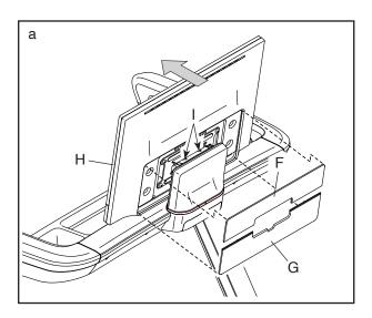
Next, tilt the top of the console (H) in the direction shown by the arrow, and use the included small hex key to tighten the two indicated M6 x 15mm screws (I) a small amount. b. Tilt the console (H) upward as shown, and use the small hex key to tighten the two indicated M6 x 15mm screws (I) a small amount, until the console no longer feels loose. Then, see the drawing at the left and
