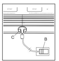
causing the walking belt to slow to a stop. Test the clip by taking a few steps backward; if the key is not pulled from the console, adjust the position of the clip.
