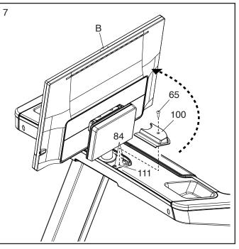
8. Rotate the console assembly (B) to the position shown.
