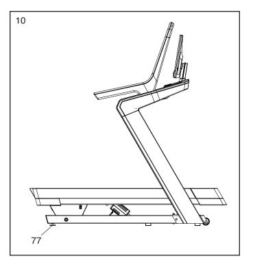
11. Make sure that all parts are properly tightened before you use the treadmill. Keep the included hex keys in a secure place. One of the hex keys is used to adjust the walking belt (see page 27). To protect the floor or carpet from damage, place a mat under the treadmill. To avoid damage to the console, keep the treadmill out of direct sunlight.
