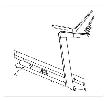
Carefully roll the treadmill to the desired location, and then lower the base to the floor.
