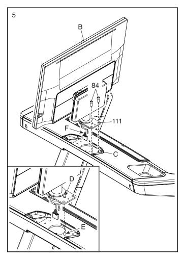
Rotate the console assembly (B) so that it faces the opposite direction. Tighten two 5/16" x 3/4" Screws (84) into the Pivot Plate (111); start both Screws, and then firmly tighten them.
