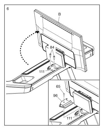
Rotate the console assembly (B) back to its original position. Firmly tighten the two 5/16" x 3/4" Screws (84) that you attached in step 5.
