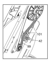
When the Drive Belt (99) is tight, reattach the parts that you removed.
