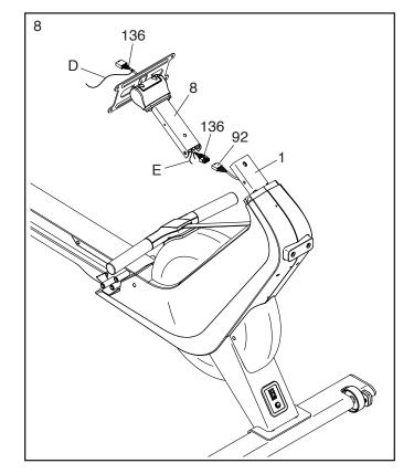
Do not pinch the wires. Attach the Neck (8) to the Frame (1) with two M8 x 16mm Screws (130), two M8 Washers (129), and an M8 x 32mm Screw (125); start all three Screws, and then tighten them.
