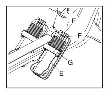
heel bracket. Then, tighten the strap (G) over your foot.
