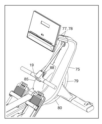
Then, remove the Upper Cover (85), the Front Cover (79), the Lower Cover (80), and the Right Shield (75). To locate the screws that attach each part, see EXPLODED DRAWING B on page 31. Note: You will need the help of a second person to tip the rower to the side to access the lower Cover.
