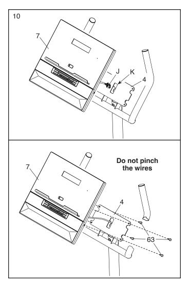
11. Connect the console wire (J) to the Main Wire (25).
